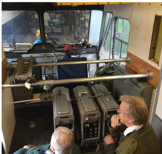
Kee Lite alloy tube was used to support the monitor stack and other electronics
