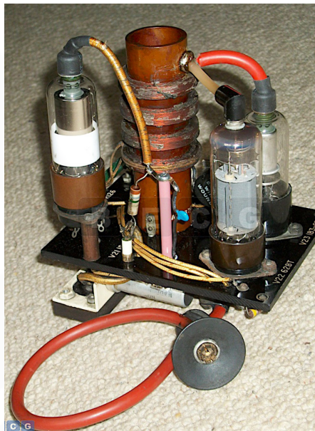
Fully restored EHT module for a Mk III picture and waveform monitor. The original Visconol oil-filled capacitors are always faulty and have been replaced
