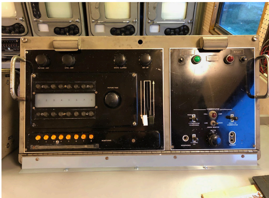
Vision mixer control panel installed in desk. Most of the electronics is in a rack
