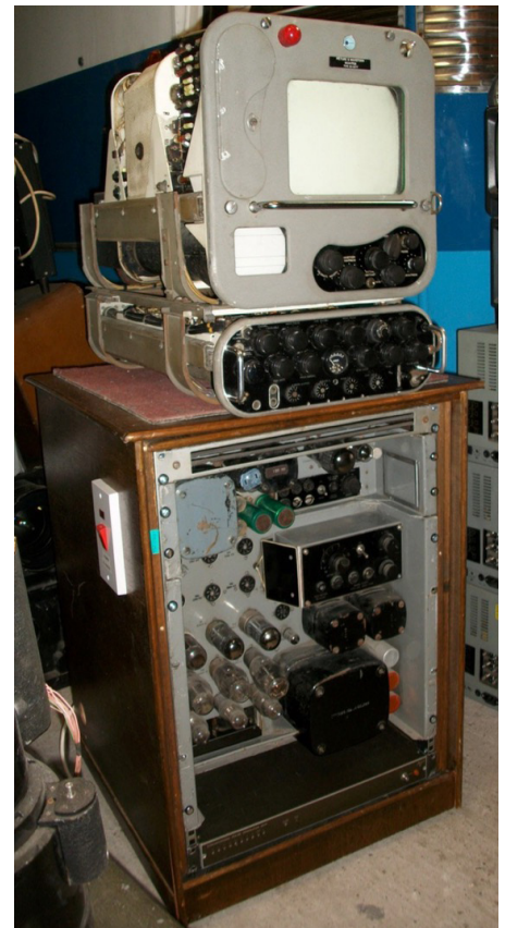
Mk III camera test rig showing a picture and waveform monitor. It's sitting on a rack with a studio-style camera control unit and modern SPG
