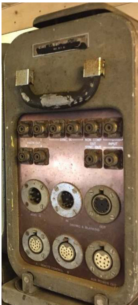
Video processing amplifier before and after restoration showing PL259 and EP connectors. Some connections are still temporary – we shouldn't have any visible cream coloured co-ax
